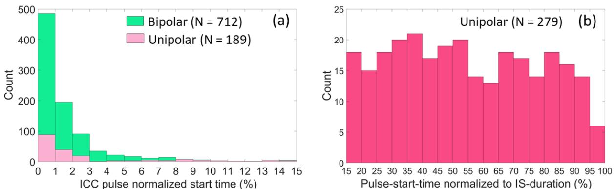
Figure 2 - Histogram of the normalized pulse-start-time for pulses occurring during (a) the IPP, color-coded in green and pink for bipolar and unipolar pulses, respectively, and (b) the MP of the IS in the 58 upward flashes in our dataset. Only unipolar pulses occur during the MP.
