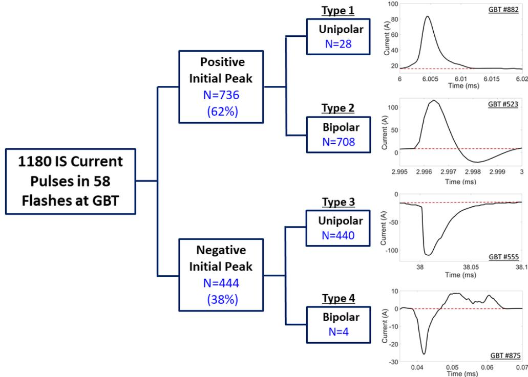
Figure 1 - Categorization of IS current pulses based on the polarity of initial peak and overall waveshape with respect to the background current. We analyzed 1180 current pulses that occurred during the IS of 58 flashes recorded at the GBT in 2006-2014. Typical current waveforms of each pulse type are shown in the rightmost panel. The red dashed line indicates the background IS current-level at the start of each pulse. Polarity of current indicates the polarity of charge transferred to ground.
