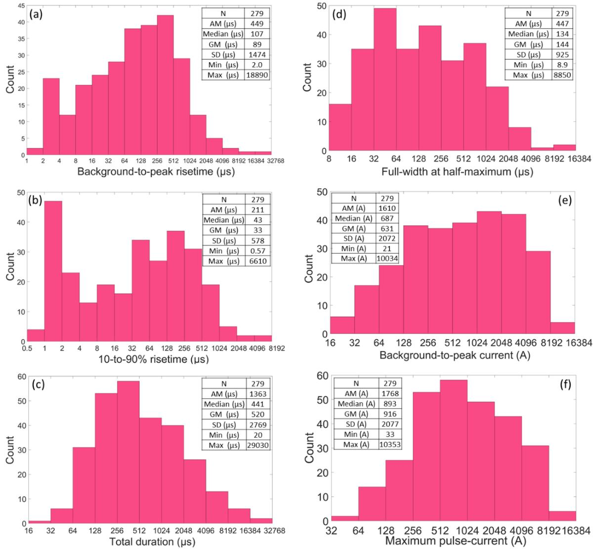
Figure 5 - Histogram of (a) background-to-peak risetime, (b) 10-to-90% risetime, (c) total duration, (d) FWHM, (e) background-to-peak current, and (f) maximum pulse-current, for unipolar pulses occurring during the MP in the 58 flashes in our dataset. Statistics are shown in each histogram.
