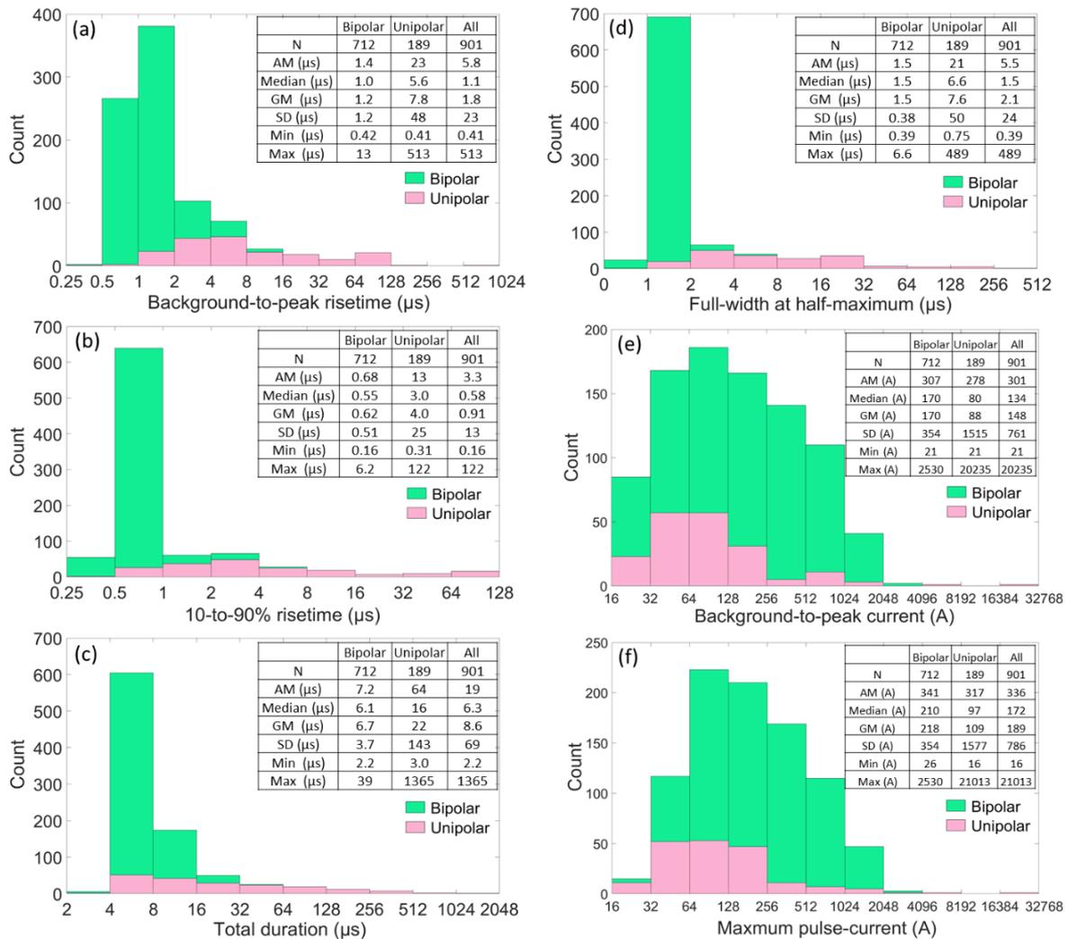
Figure 4 - Histogram of (a) background-to-peak risetime, (b) 10-to-90% risetime, (c) total duration, (d) FWHM, (e) background-to-peak current, and (f) maximum pulse-current, color-coded in green and pink for bipolar pulses and unipolar pulses, respectively, occurring during the IPP in the 58 flashes in our dataset. Arithmetic mean (AM), geometric mean (GM), maximum (Max), and minimum (Min) values for bipolar, unipolar, and all pulses are shown in each histogram.
