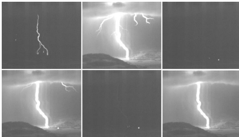
Figure 5: Stepped leader, first return stroke (FI1), flashover on two towers, subsequent stroke 2 (SU1), flashover on three towers and subsequent stroke 3 (SU1) from top left to bottom right; © LiOn IHS TU Graz 2019
