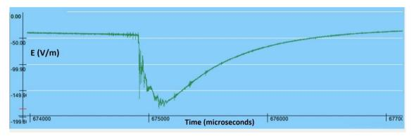
Figure 7. Electric field sensor and the signature of a lightning stroke.
