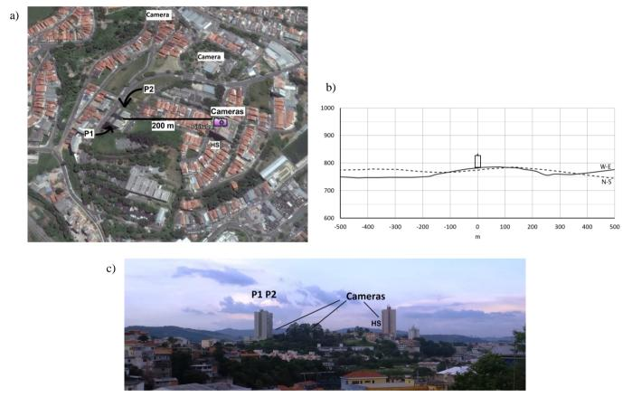
Figure 2. . a) Location of the twin buildings P1, P2 and cameras; b) approximate elevations (m) of the terrain along two directions: West to East (solid line) and North to South (dashed line), taken from Google Earth. The building is drawn on W-E elevation curve in scale; c) a side view of buildings P1, P2, HS and the location of the cameras.
