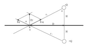
Figure 1: Image Method for Charge Transfer (adapted from [7])
