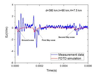
Fig. 5. FDTD simulations of the electomagnetic fields at 380 km, taking into account the ionospheric reflections and comparison with measured waveform.
