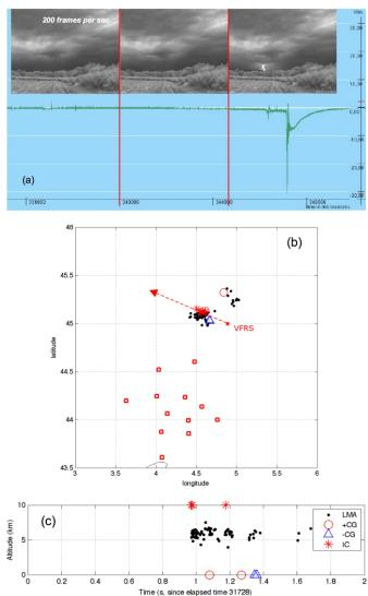
Fig.3: Example of concurrent observations during 2 seconds with (a) observations collected by the VFRS during the first stroke of the negative cloud-to-ground flash, (b) ground projections of the strokes as located by EUCLID as well as the VHF sources simultaneously located by LMA, (c) time-height of the HyLMA sources as well as times of EUCLID records with IC records set to an arbitrary altitude of 10 km.
