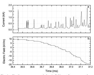
Fig. 6. Simultaneous current and electric field waveforms measured at a distance of 170 m from the GBT for the flash GBT #482, illustrating the high repetition characteristics of current pulses at the initial portion of initial stage current of the upward positive flash.
