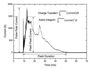
Fig. 1. Measured lightning current waveform (GBT # 380) illustrating the definitions of current parameters (pulse peak current, flash peak current, flash duration, charge transfer, and action integral) for upward positive lightning flashes.
