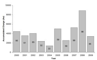
Figure 2 – Accumulated charge transfer per year measured at the GBT (2000 – 2009). Numbers in the bars indicate the number of flashes contributing to the total annual charge
