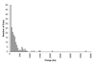
Figure 4 – Distribution of charge transfer per on-site thunderstorm day observed at the GBT (2000 – 2009)
