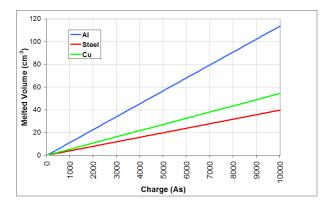
Figure 5 – Estimated melted volume as a function of charge using Eq.(1) for material AI, Steel, and Cu assuming  $u_{\rm a,c}$  = 30V,  $\theta_{\rm u}$  = 20°
