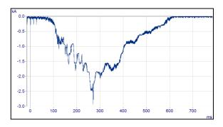
Figure 1 – Current record of flash # 614 with a transferred charge of 546 As
