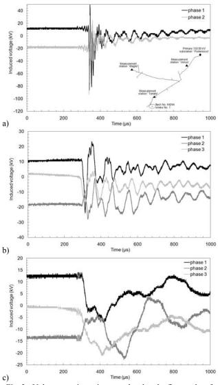
Fig. 2 - Voltage transients time correlated to the first stroke of lighting flash #64244 measured at the three substations: a) Torrate (only phase 1 and phase 2 are available), b) Venus, and c) Maglio.
