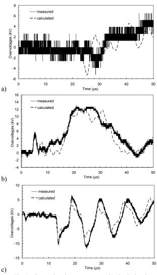
Fig. 5 – Comparison between measured and calculated overvoltages in phase 2 at the three substations: a) Torrate, b) Venus, c) Maglio, for stroke 30260-4. Stroke location and current peak amplitude using the best matching procedure.
