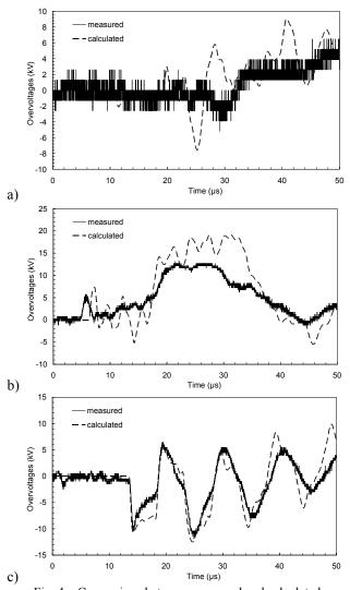
Fig. 4 – Comparison between measured and calculated overvoltages in phase 2 at the three substations: a) Torrate, b) Venus, c) Maglio, for stroke 30260-4. Stroke location at the centre of the error ellipse and current peak amplitude equal to the LLS estimation.
