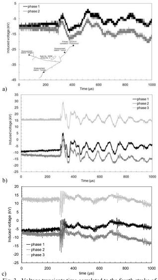
Fig. 3 - Voltage transients time correlated to the fourth stroke of lighting flash #30260 measured at the three substations: a)
