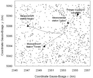
Fig. 1 – Considered distribution feeder, LLS-detected stroke locations during the period March 2007 – August 2008, position of measurement stations and of the primary substation.
