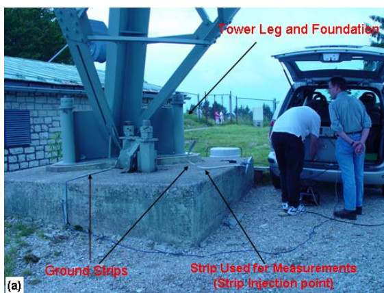
Figure 1: (a) The buried grounding strips taking from one of the tower legs. Also shown is the ground strip on which the currents were measured (b) The three measurement points along the grounding strip; I_0 is measured at the injection point (0 m at location A), I_1 and I_2 are measured at distances 40 m (location B) and 60 m (location C) from the injection point.
