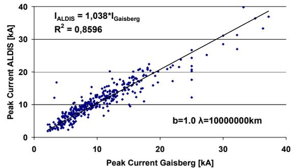
Fig. 3: Comparison of peak current measurements at the Gaisberg tower with peak currents of correlated strokes reported by ALDIS (distance less than 2km to the tower).
