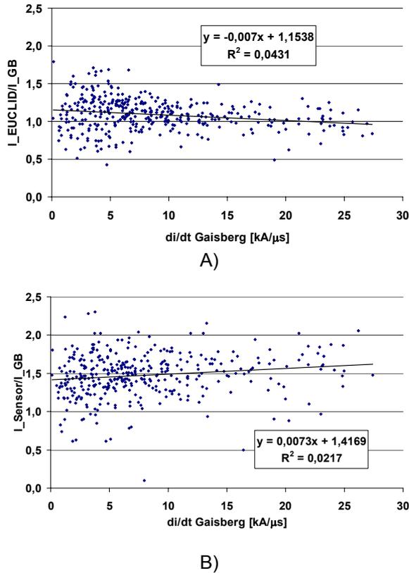
Fig. 3: Enhancement versus di/dt measured at the Gaisberg tower for peak currents inferred from A) all EUCLID sensors and B) peak currents inferred from sensor 1 data only (both calculated with a signal normalization factor of 0.23 and without attenuation parameters)
