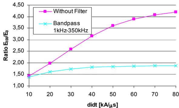
Fig. 2: Field enhancement for a 100m high tower ( $v_{rs}=1.3e8$  m/s,  $\tau_{bd}=0.3\mu s$ )
