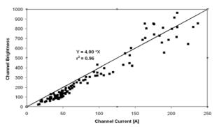
Fig.6: Brightness versus current data for line #2 in Fig.5
