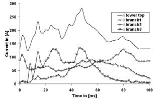
point at the tower top. During the first few milliseconds current flows almost only in branch 3 and branch 1 and 2 inject a first current peak after about 8 and 15 milliseconds, respectively. A MPEG movie that we have generated from the full set of BMP images provide a good visual impression of these changes in the current distribution among the visible branches.
