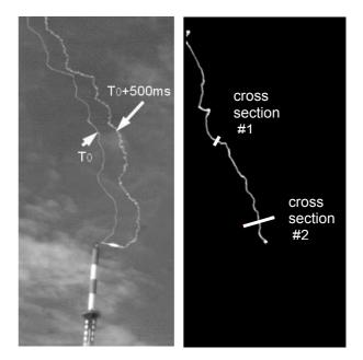
Figure 4: Overlay of two lightning images separated in time 14<sup>th</sup>, 2000 20:19:52 by 500 ms to demonstrate the wind shift of the lightning channel
