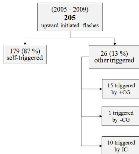
Fig. 15. Classification of self-triggered and other-triggered flashes to the GBT from 2005 to 2009 (adopted from [13]).
