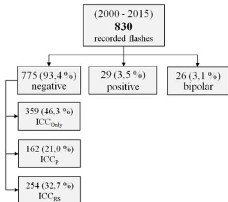
Fig. 6. Occurrences of the various types of upward initiated discharges at the GBT for the period 2000 - 2015
