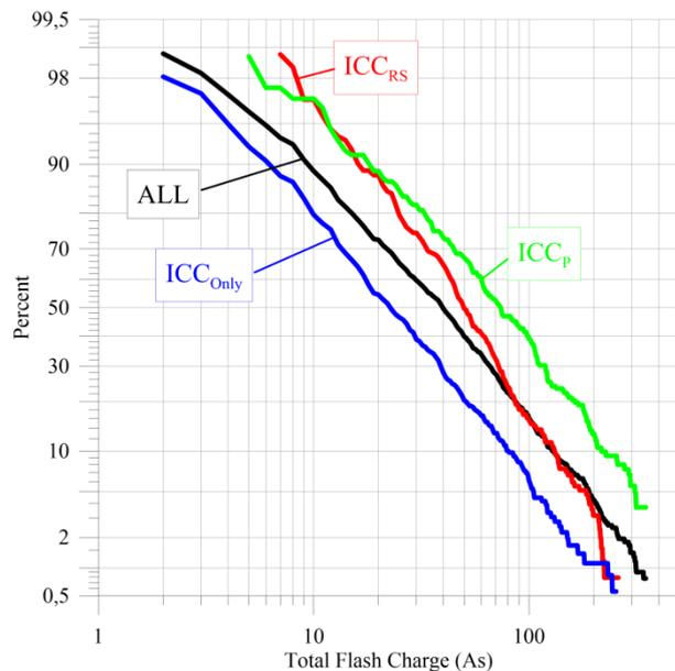
Fig. 8. Log-normal plot of total charge transfer per flash for the three types of flash currents in upward initiated discharges
