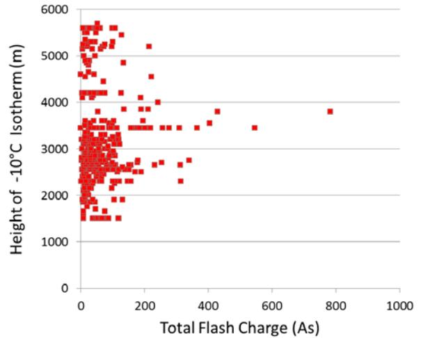
Fig. 14. Height of -10° C Isotherm was determined by the mean height obtained from the last radio sounding prior and after the occurrence time of the recorded flash at the GBT
