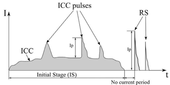
Fig. 1. Schematic current record for an upward-initiated flash. The initial stage (IS) is characterized by ICC with superimposed ICC pulses. The IS is followed by two RS after a period of no current flow.
