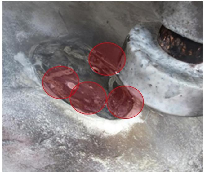
Fig. 6. Melting effect of long duration current with the charge of 300 As and the duration of  $t=0,5$  s
