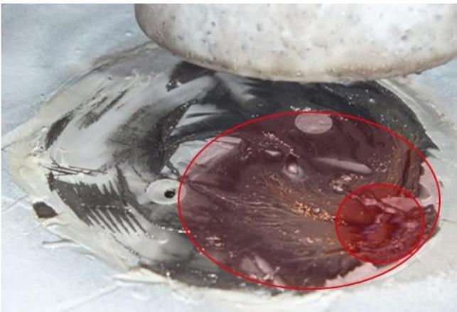
Fig. 5. Melting effect of an 200 kA 10/350  $\mu$ s impulse current test
