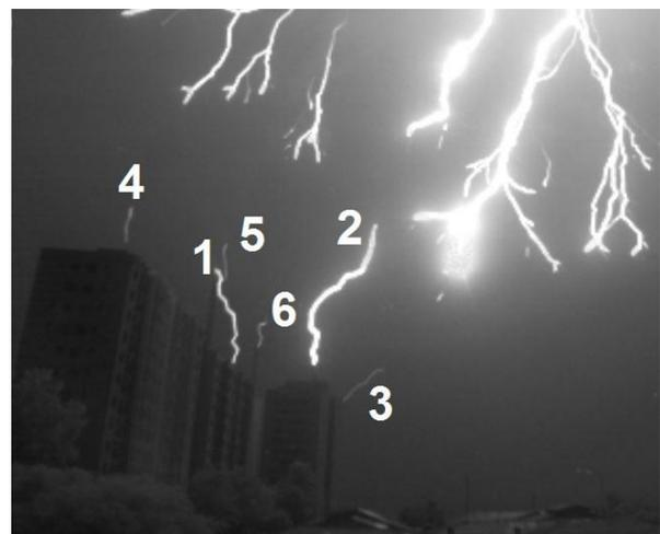
Fig. 3 – UCL from P2 (number 2), and UULs (numbers 1, 3, 4, 5 and 6) from the mast of P1, the side of P2, and from other buildings nearby (see Fig. 1).
