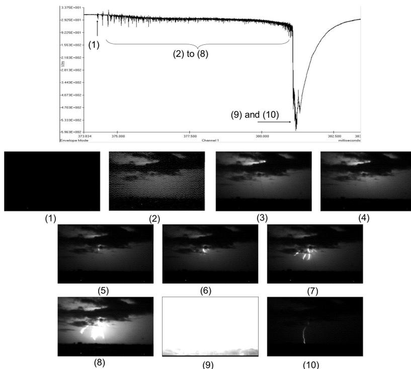
**Figure 1.** Correlated fast electric field measurements (top) and high-speed camera frames (bottom) of a negative stepped-leader. The time interval between each frame is 1 ms.
