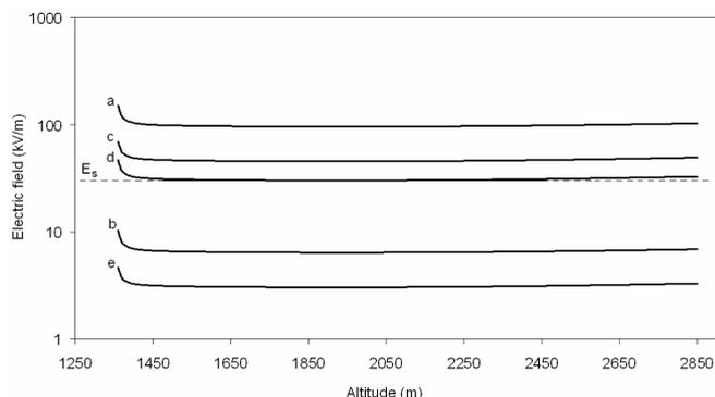
Figure 4. Electric field along the vertical axis of the tower. *a* and *b* correspond to winter cloud structure with 3 and 0.2 nC m<sup>-3</sup> cloud charge densities, respectively. *c*, *d* and *e* correspond to summer cloud structure with 3, 2 and 0.2 nC m<sup>-3</sup> cloud charge densities, respectively.  $E_s$  is the stabilization electric field.
