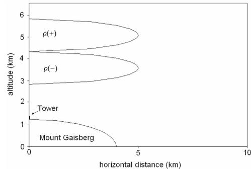
Figure 3. Geometry used for electrostatic simulations (case of winter).
