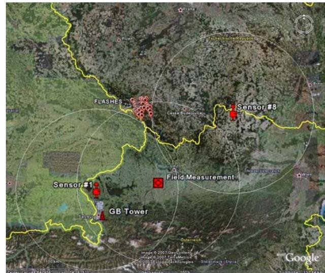
Fig. 2: Location of selected lightning flashes relative to ALDIS sensor #1 and sensor #8 and to the Field measurement site in Wels. Circles show 100 km distance range around the sensors and the field antenna.
