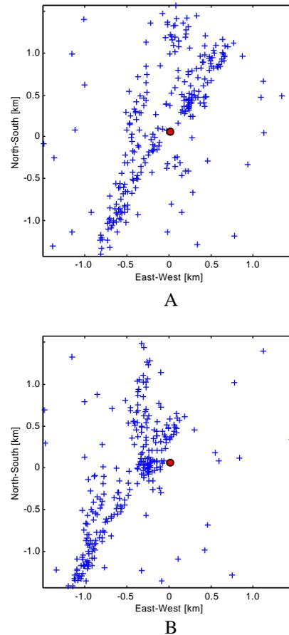
**Figure 1.** Flashes around Dobratsch before (A) and after (B) implementation of a 2 x 2 arc minute elevation model
