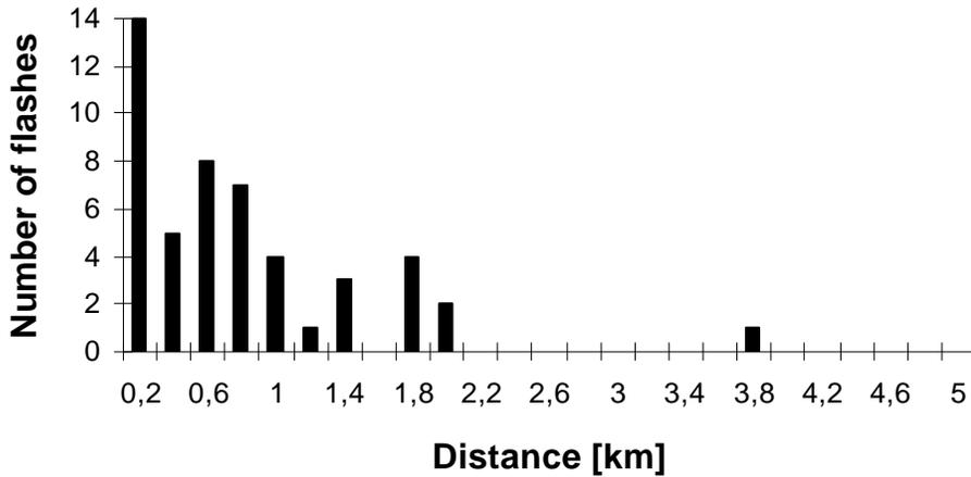
Fig. 5: Perpendicular distances of location of flashes time correlated with power line outages to the power lines (1995)
