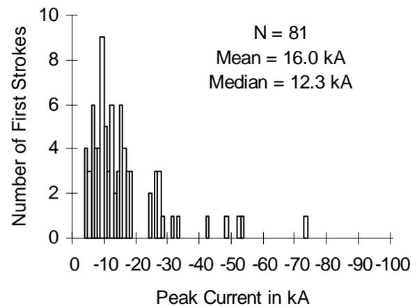
Fig. 2a: Peak current distribution for first strokes located in an area of  $0 \text{ km} < R < 1 \text{ km}$  around the tower position
