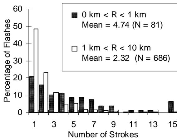
Fig. 3: Number of strokes per flash around the Gaisberg tower
