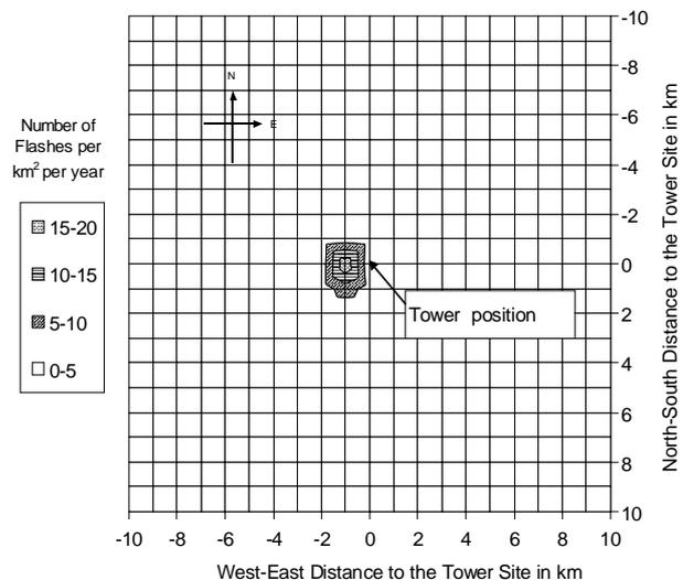
Fig. 1: Lightning flash density in the area of the Gaisberg tower (47.8047°N / 13.11056°E, 1288 m above sea level)
