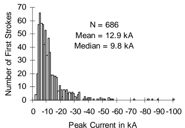
Fig. 2b: Peak current distribution for first strokes located in an area of  $1 \text{ km} < R < 10 \text{ km}$  around the tower position
