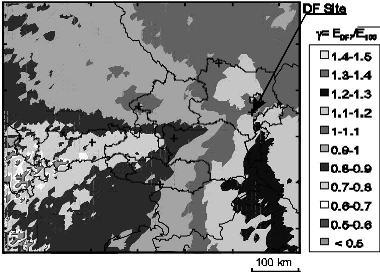
Fig. 6: Contour plot of the ratios  $\gamma_7$  for DF 7 in the Austrian lightning location network ALDIS
