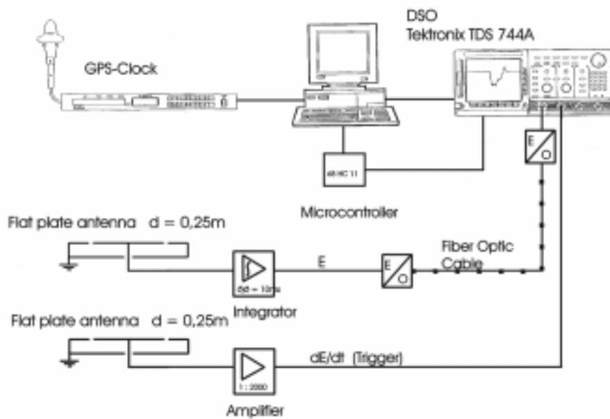
Fig. 7: Experimental setup used for field measurements in Austria and Florida
