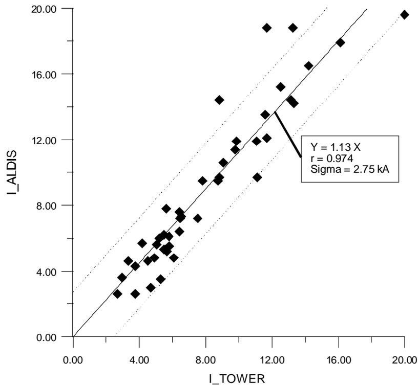
Fig. 2: Scatter plot of measured stroke peak current versus peak current reported by ALDIS (dashed lines represent the plus/minus sigma region)
