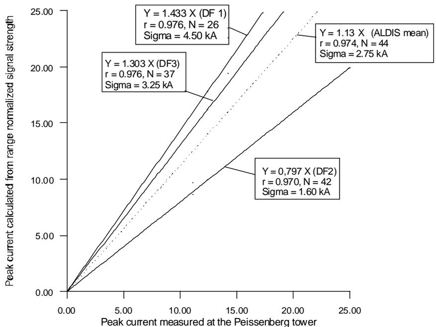
Fig. 3: Regression lines fitted to the range normalized data of the three closest DF of the Austrian network to the Peissenberg tower
