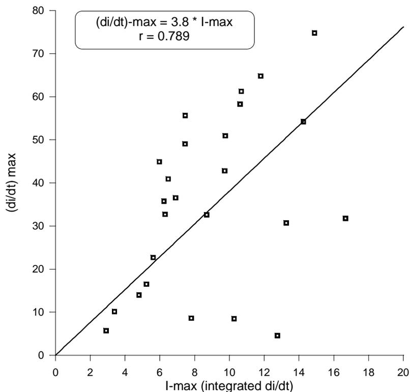
Fig. 4: Scatter plot and regression line for the peak current  $I_{max}$  in kA integrated from  $(di/dt)$  versus the maximum current derivative  $(di/dt)_{max}$  in kA/ $\mu$ s.
