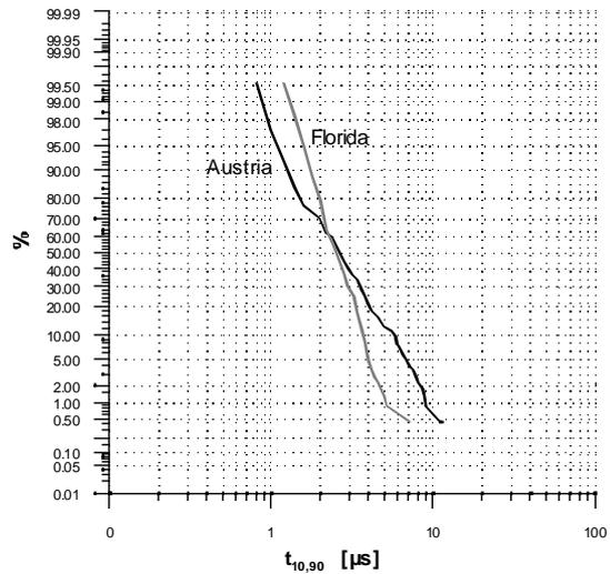
Fig.9: Rise times of subsequent strokes
