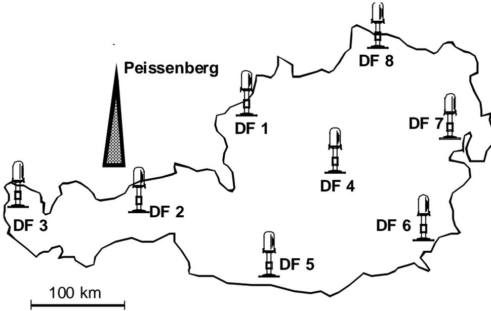
Fig. 1: Sites of IMPACT sensors in Austria and location of the Peissenberg tower
